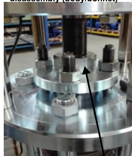
The gag iron nut used to keep the spring pressed for safety valve disassembly (body/bonnet)
