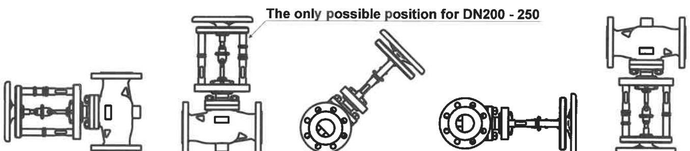
Installation position for valves with hand wheel
