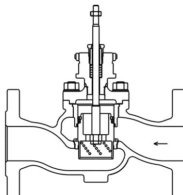
Pic.2: Flow direction for valve with perforated plug
