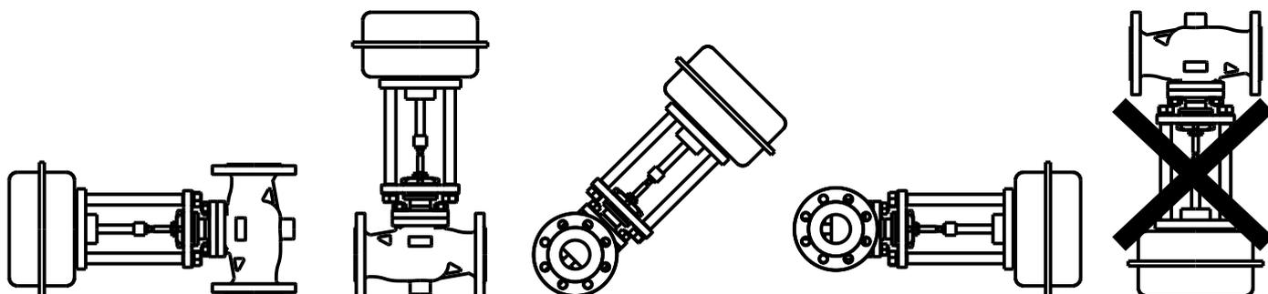
Pic. 3: Installation position for valves with electro- or pneumatic actuators
