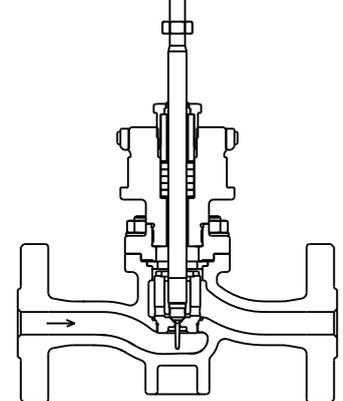
Pic.1: Flow direction for two-way valve with V-ported or contour plug
