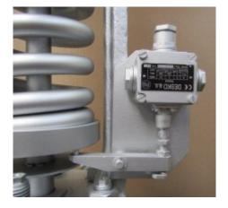
lift indication – micro switch/signal lamp/electric circuit
