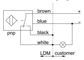
safety valve closed - the signal lamp is OFF safety valve open - the signal lamp is ON
