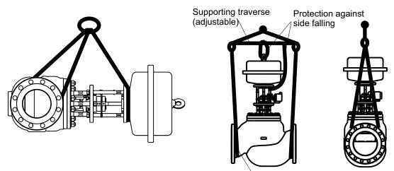
Example of lifting device usage.
