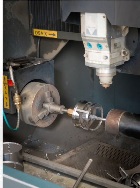
Laser Cutting of V-ported plugs
